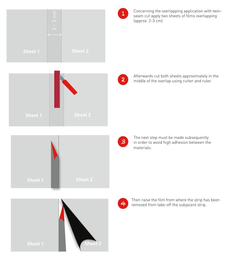
Repeat steps 1-4 (orders 5) for any additional sheet/layer we recommend to rework the whole application with high pressure.
